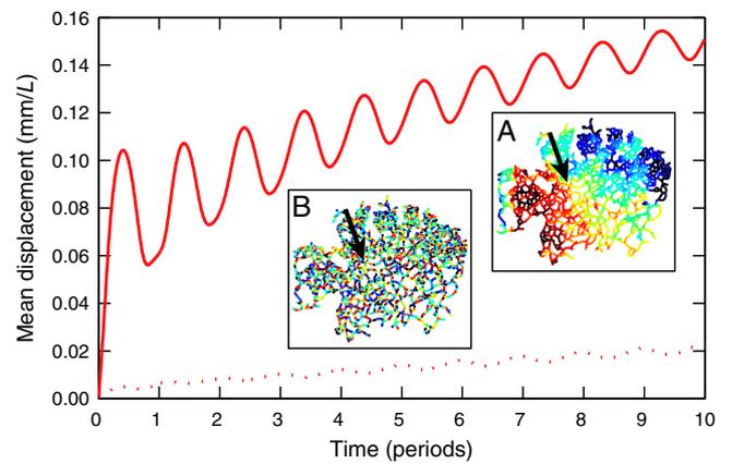
**Fig. 4.** Networks optimized for minimal local phase difference maximize particle transport. Numerically calculated mean displacement of tracer particles within the large real *P. polycephalum* network architecture of Fig. 3A is shown here for theoretically optimized (*Inset A*, solid line) and random (*Inset B*, dashed line) phase patterns. The mean displacement is normalized by the largest distance  $L$  in the network. Arrows mark the site of tracer initiation.
